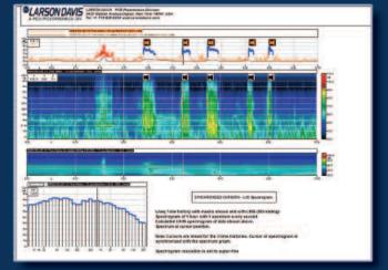
**Fig. 21** DNA Software — TH with embedded .wav files on event, color spectrogram, L<sub>95</sub> and 1/3 octave frequency analysis.
