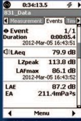
Fig. 22 Event Detection Display on Model 831
